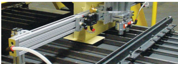
(2) Model 6083 1-1/2" (38mm) Line Vacs convey rejected metal caps from a fluorescent lamp operation to a scrap bin.
