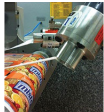
1" (25mm) Line Vacs remove and discard a label matrix.
