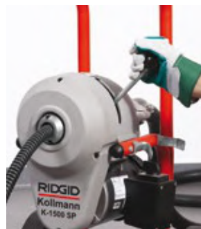
Engage clutch, cable spins
