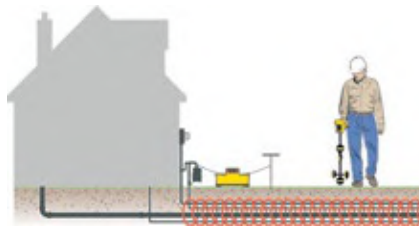
Direct connect to utility lines.
