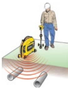
Induce a signal to locate utilities.
